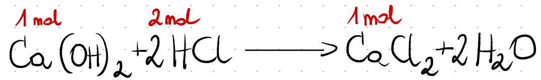
$$\begin{array}{ll} V=1 \text{ L} & m=7.41 \text{ g} \\ \text{at } 25^\circ\text{C} & m=7.23 \text{ g} \\ M_{\text{Ca(OH)}_2}=74 \text{ g/mol} & M_{\text{HCl}}=36.5 \text{ g/mol} \\ n=0.1 \text{ mol} & n=0.2 \text{ mol} \end{array}$$
